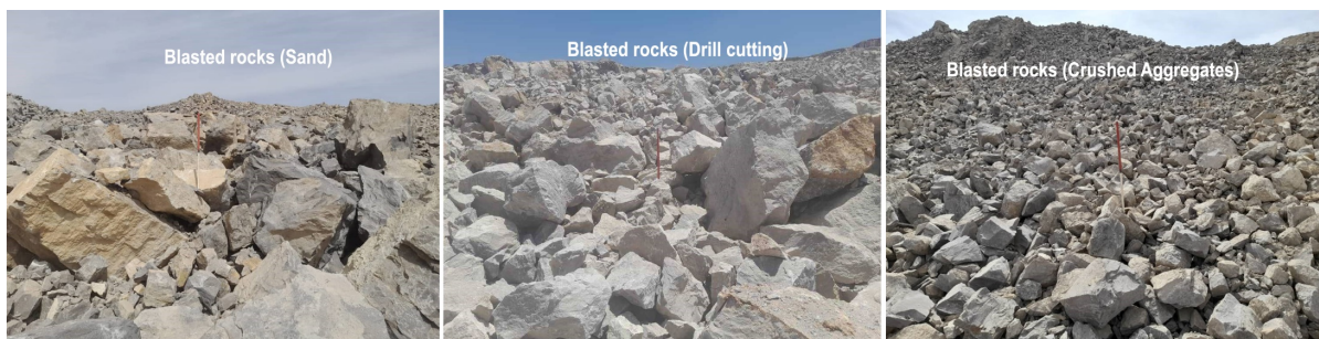
Figure 5. Photos of the blasted rocks taken for each of the stemming materials after blasting
