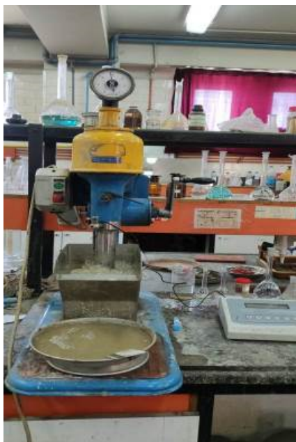
Figure 1. Denver laboratory flotation cell used
