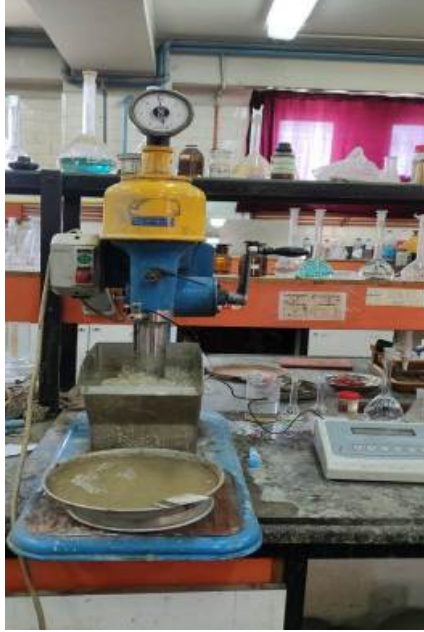
Figure 1. Denver laboratory flotation cell used
