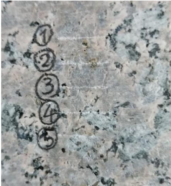
Figure 5. Scratched appearance of stone sample after five tests
