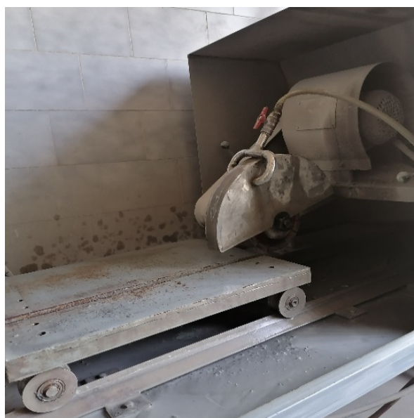
Figure 6. A view of circular sawing machine used in this study to measure SW
