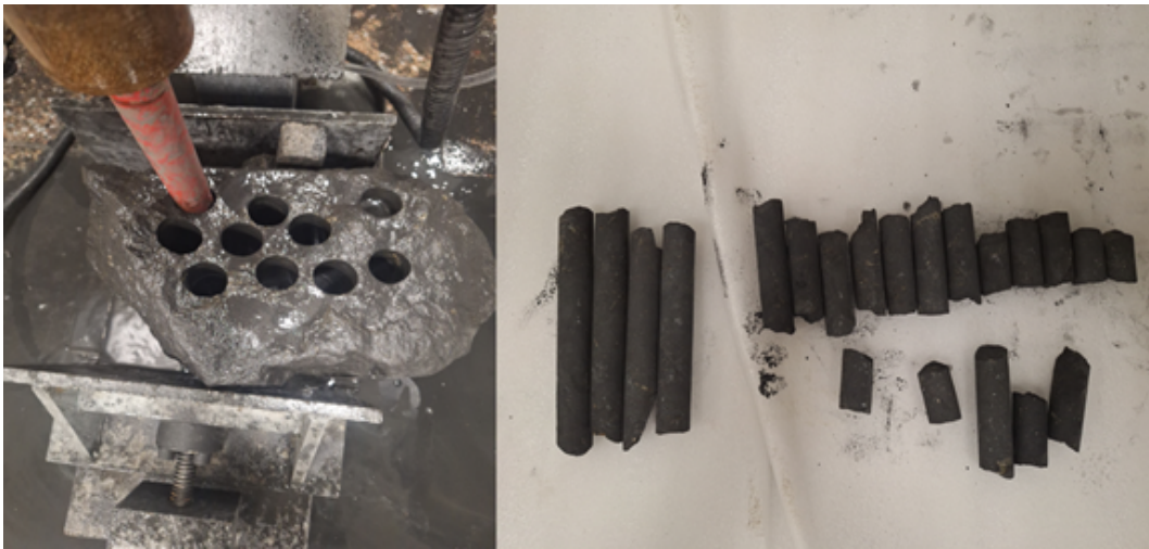
Figure 2. Core drilling process and extracted iron ore core samples
