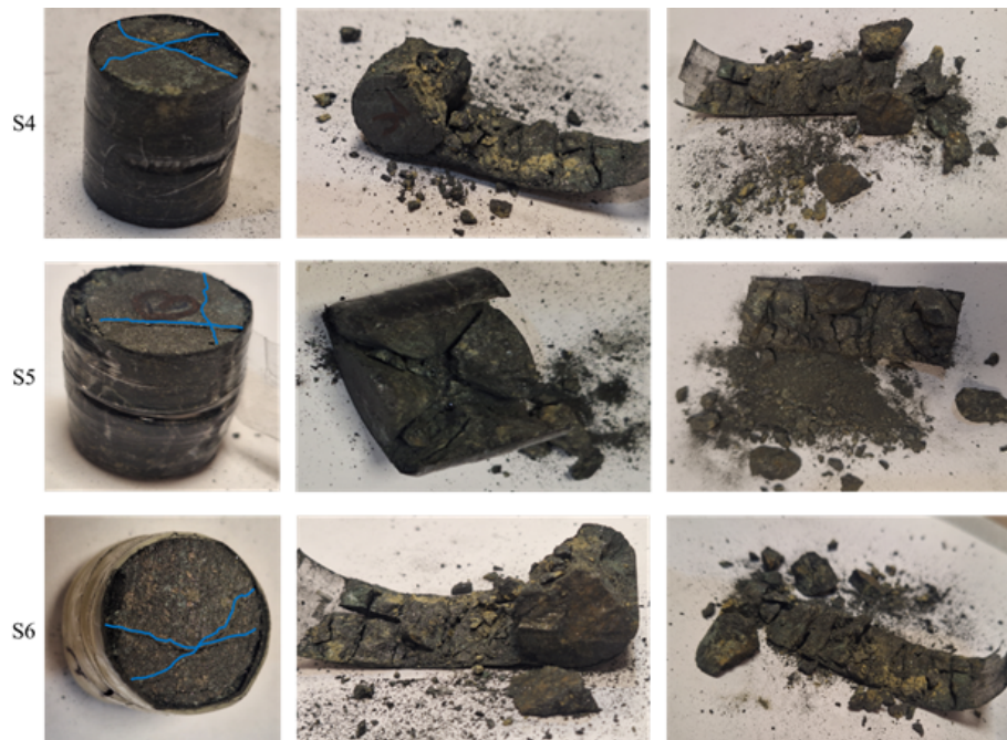
Figure 11. Failure patterns of specimens with a notch inclination angle of 0^\circ and a notch position at L/2 of the specimen length relative to the incident bar: (S4) notch surface/ total shear surface = 0.2; (S5) notch surface/ total shear surface = 0.4; (S6) notch surface/ total shear surface = 0.6.
