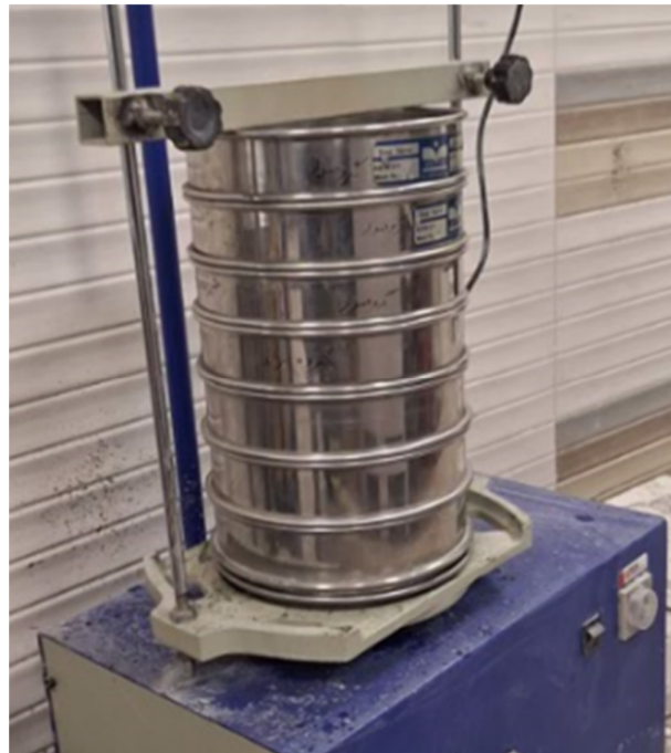
Figure 13. Grading sieves used for fragment size analysis after impact crushing.
