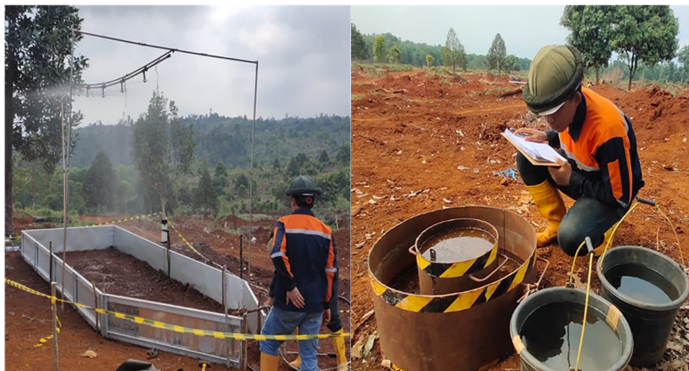
Figure 3. Erosion and infiltration test activity
