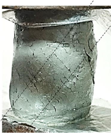
Figure 35. Actual specimen after uniaxial compression loading
