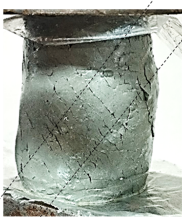
Figure 35. Actual specimen after uniaxial compression loading
