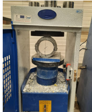
Figure 3. Axial loading test.
