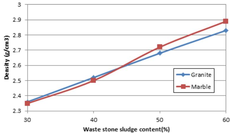
Figure 4. Effect of sludge content on density.
