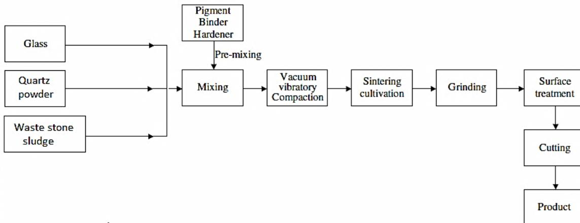
Figure 3. Manufacturing procedure of artificial stone slabs.
