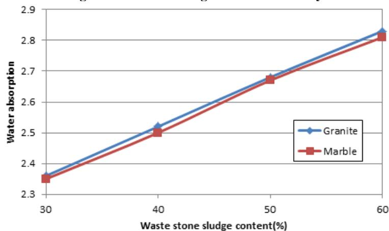
Figure 5. Effect of sludge content on water absorption.
