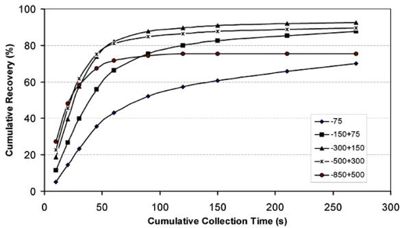
Figure 1. Cumulative recovery of different fractions of coal particles against flotation time
