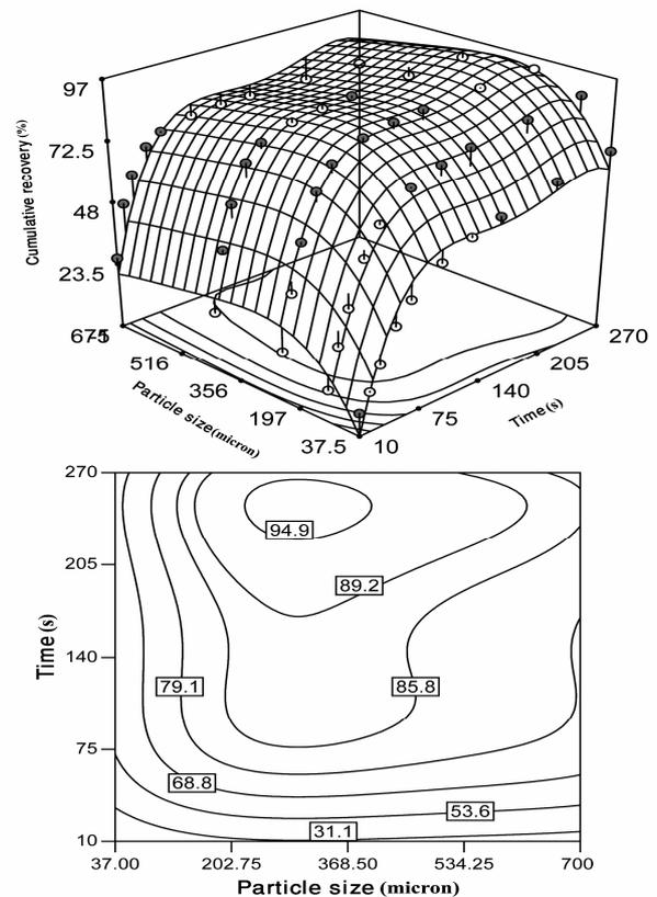
Figure 5. Response surface and contours for the cumulative recovery
