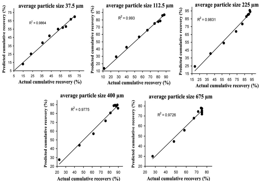
Figure 6. Comparison between actual and predicted cumulative recoveries for individual size fractions
