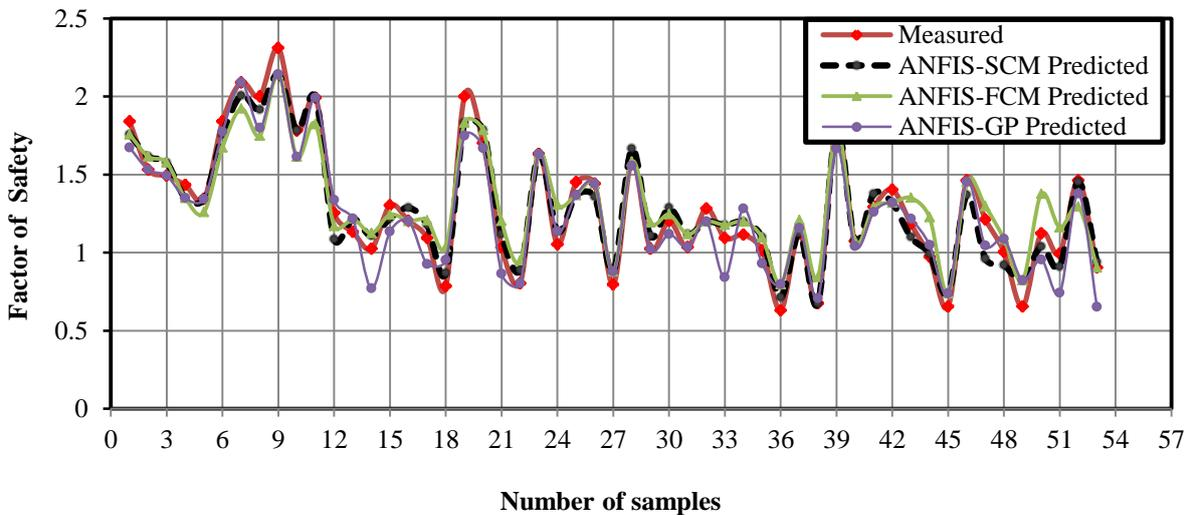
Figure 9. Comparison between measured and predicted FOS by ANFIS models for training datasets.
