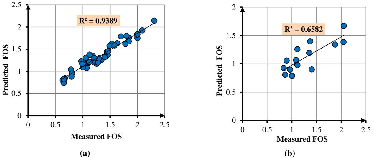
Figure 7. Correlation between measured and predicted FOS values by ANFIS-FCM model: a) training data, and b) testing data.
