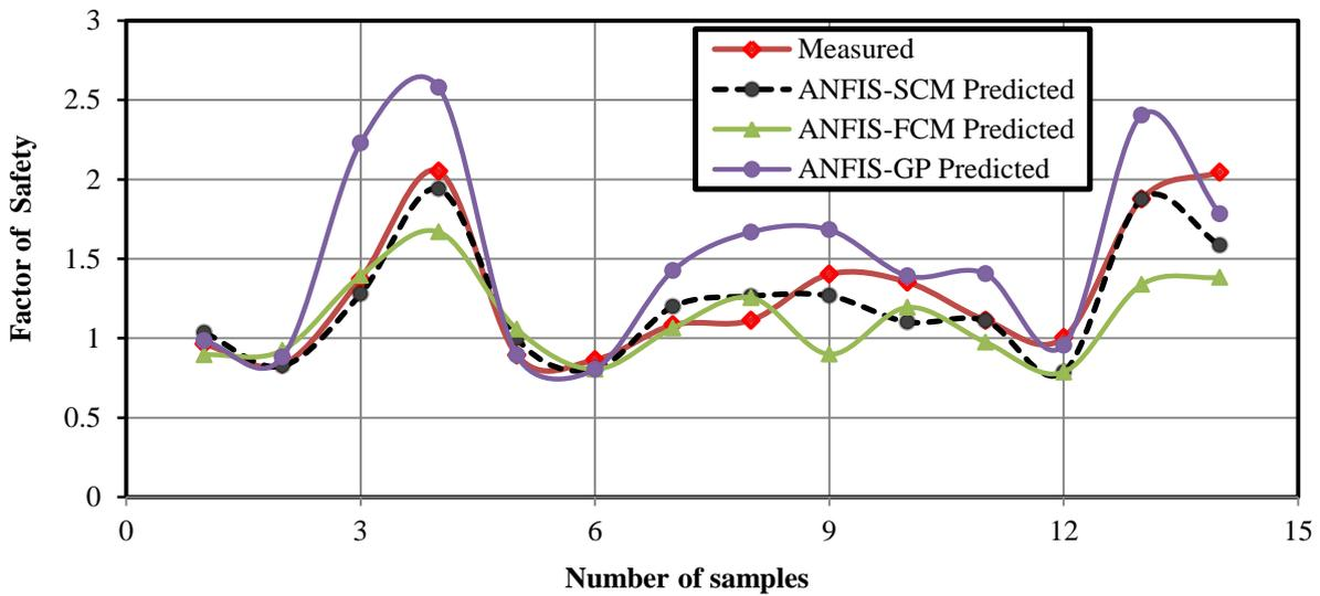
Figure 8. Comparison between measured and predicted FOS by ANFIS models for testing datasets.
