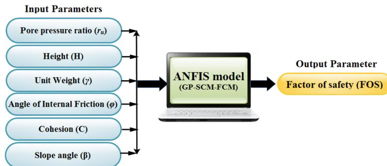
Figure 1. Architecture of ANFIS based on GP, SCM, and FCM.
