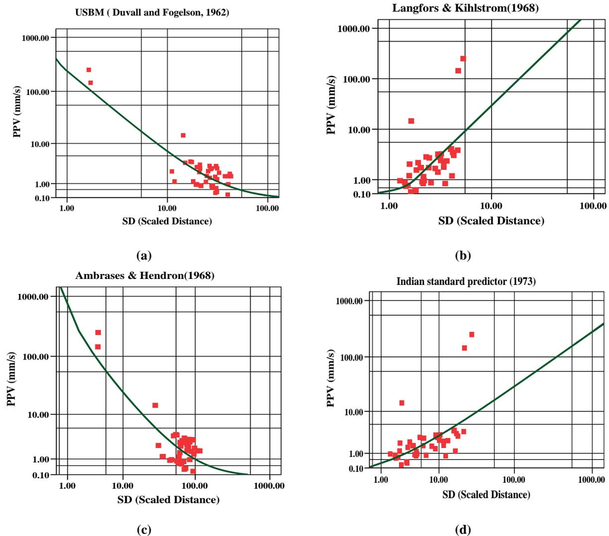
Figure 9. PPV prediction based on different predictors listed in Table 3 for extended database. a) USBM, b) Langfors & Kihlstrom (1968), c) Ambrases & Hendron (1968), and d) Indian standard.
