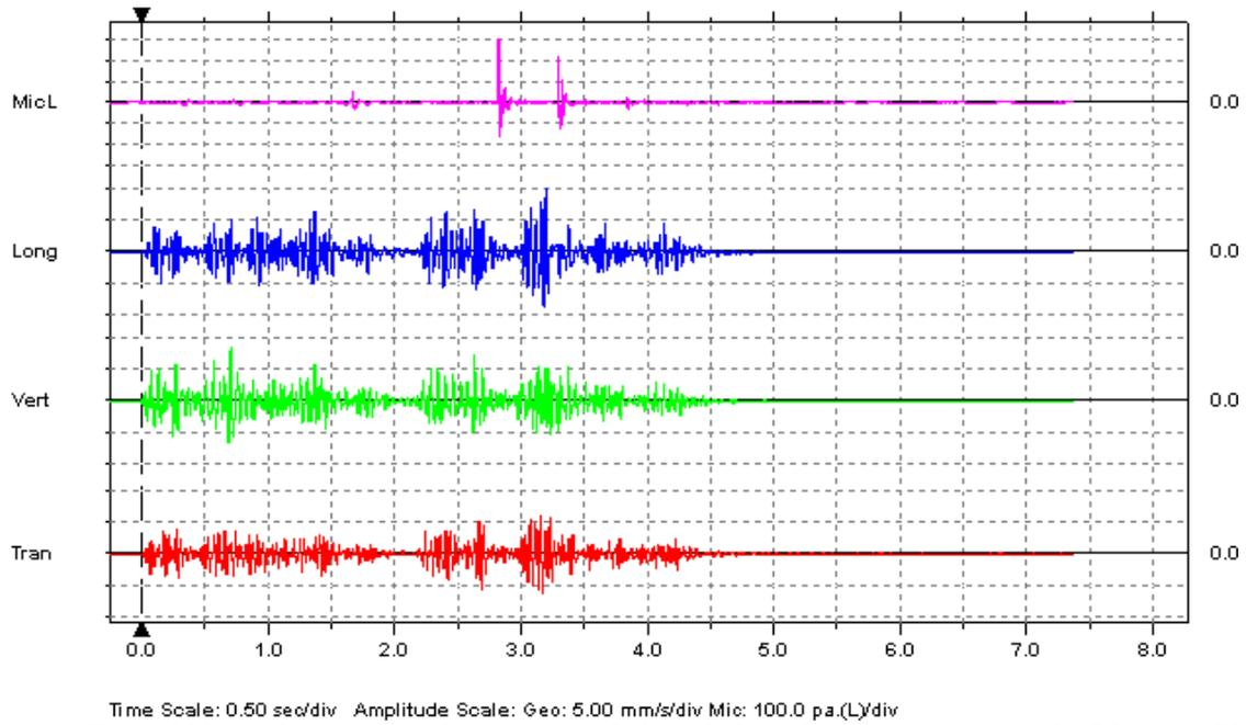
**Figure 4.** Typical blast vibration time history recorded in Shahrood Cement Company by MinimatePlus seismograph (T6.22 mm/s, F24.7 Hz; V8.51 mm/s, F24.4 Hz; L10.0 mm/s, F30.1 Hz).
