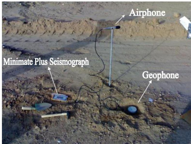
Figure2. Setup of Minimate Plus seismograph.
