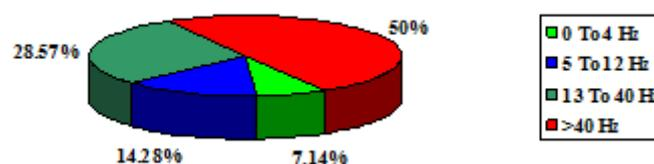
**Figure 3. Frequency distribution resulting from Shahrood Cement Company blasting based on USBM standards.**
