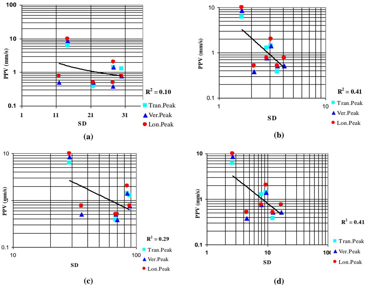
Figure 8. PPV prediction based on different predictors listed in Table 3 for recorded data in Shahrood Cement Company. a) USBM, b) Langfors & Kihlstrom (1968), c) Ambrases & Hendron (1968), and d) Indian standards.
