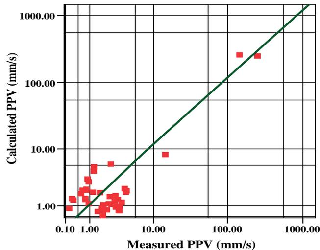
Figure 10. Correlation between PPV calculated by general formula and measured PPV.
