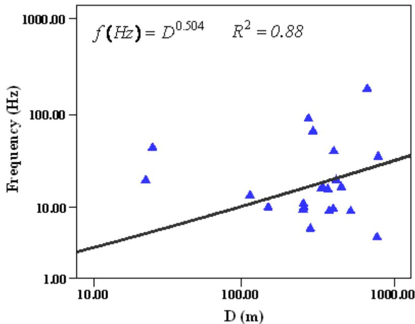
Figure 7. Frequency vs. distance from blast site.
