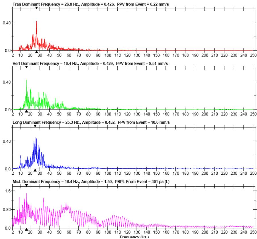
**Figure 5.** FFT analysis of frequencies of vibration recorded in Shahrood Cement Company limestone mine (dominant frequencies for Mic, T, V, and L are 16.4, 25.3, 16.4 and 26.8 Hz, respectively).
