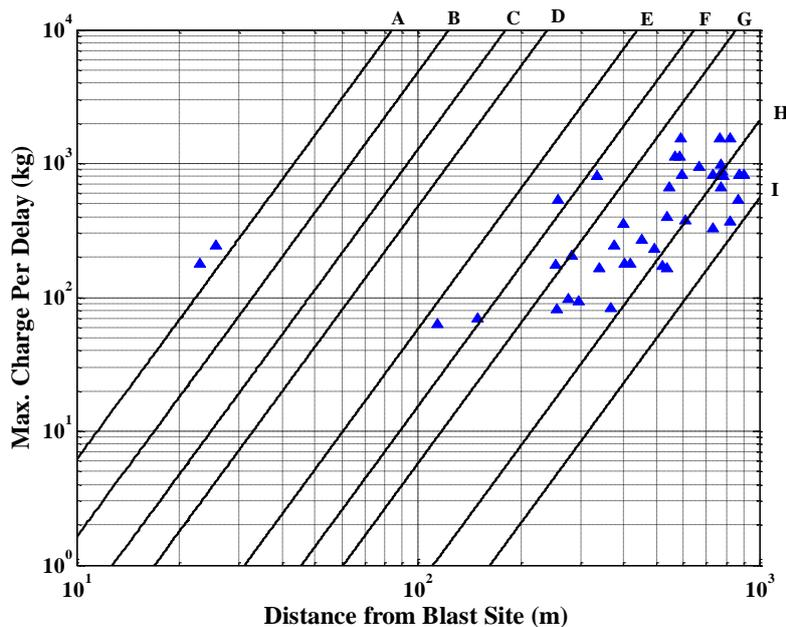
Figure 11. Prediction of maximum charge per delay based on based acceptable level of PPV and distance form blast site (A=200 mm/s, B=100mm/s, C=50mm/s, D=30mm/s, E=10mm/s, F=5mm/s, G= 3mm/s, H=1 mm/s, and I=0.5 mm/s).
