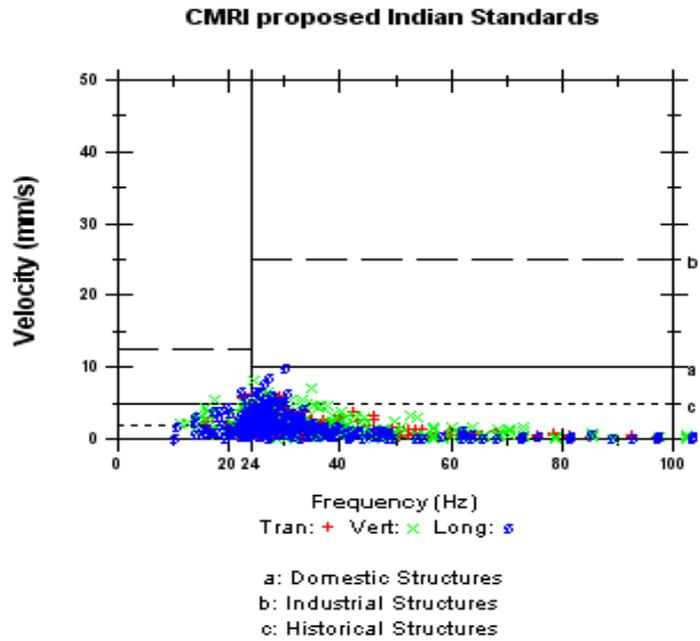
Figure 6. Acceptable level of blast-induced vibration velocities for typical FFT analysis shown in Figure 5 based on OSMRE and CMRI proposed Indian standards [22].
