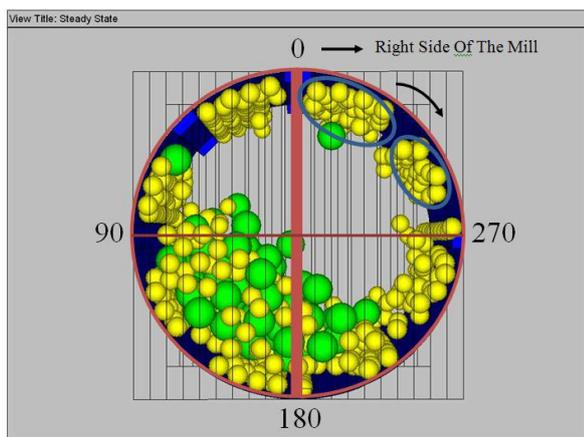
Figure 5. An example for balls movement regime in the mill including 8 lifters with 8 mm height
