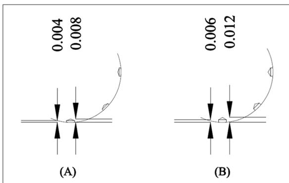
Figure 6. (A) Combination of lifters with 4 and 8 mm height; (B) Combination of lifters with 6 and 12 mm height
