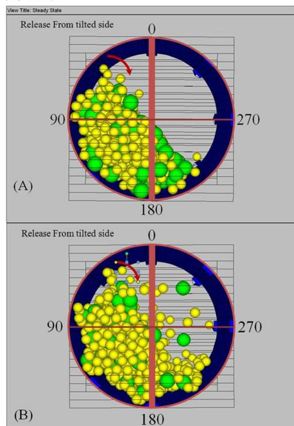
Figure 7. (A) Cascading flow in mill with 8 lifters which have 8 mm height; (B) Cataracting flow in mill with 8 lifters which have 12 mm height.
