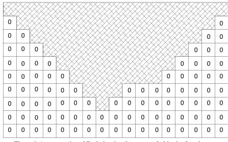
Figure 4. A cross section of final pit using the suggested objective function
