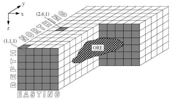
Figure 1. An example of a 3D block model for ultimate pit limits determination [1]
