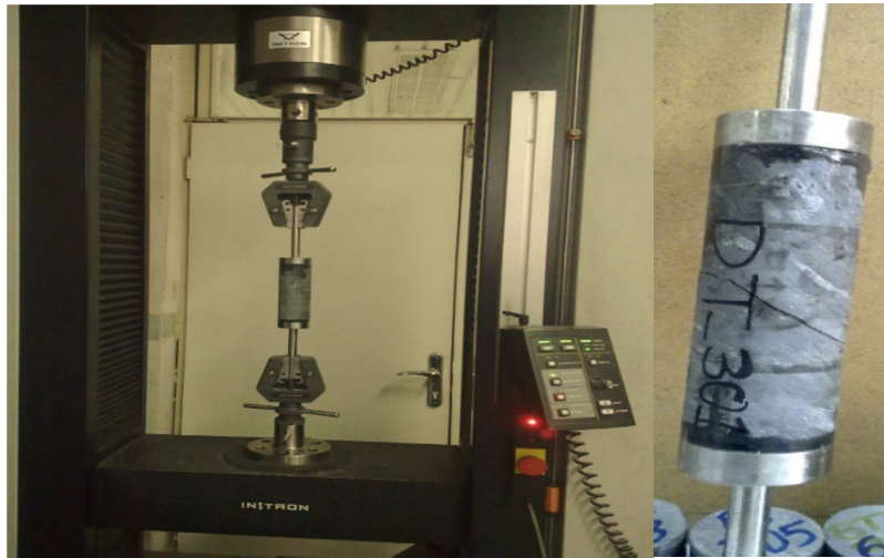
Figure 1. Servo-electric load frame and phyllite specimen.
