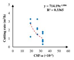
Figure 13. Correlation between  $CSF_a$  (Table 5) and cutting rate.
