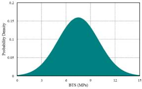
Figure 4. Normal distribution function used for Brazilian tensile strength.
