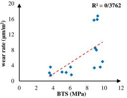
Figure 1. Linear relation between measured wear rate and BTS.
