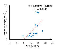
Figure 10. Correlation between *MF* (Equation 10) and wear rate.
