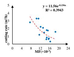
Figure 14. Correlation between *MF* (Equation 10) and cutting rate.
