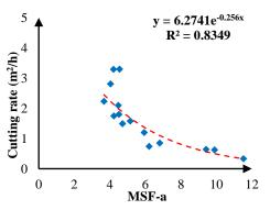
Figure 15. Correlation between  $MSF_a$  (Equation 9) and cutting rate (present study).
