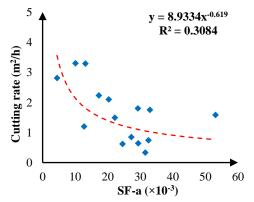
Figure 12. Correlation between  $SF_a$  (Equation 1) and cutting rate.
